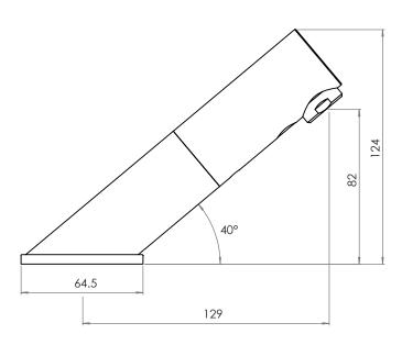
Every effort is made to ensure specifications are correct at the time of printing. Autoflo Pty Ltd reserves the right to make changes without prior notice. All measurements shown are in millimetres.
